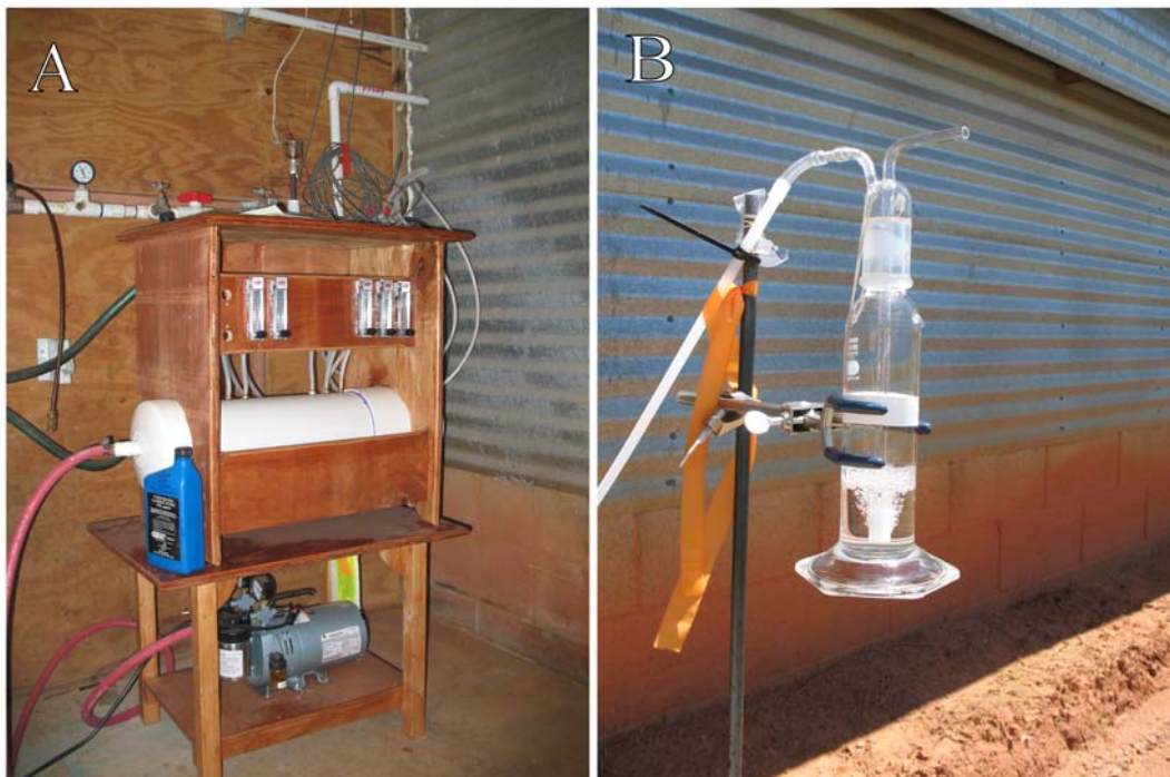
Fig. 1. Gas washing technique. Fig. A is the pump and control system for the gas washing bottle (B).
